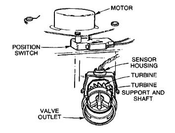
**B.** The letter (P) and dash (or dashes) indicate POSITION switch operation. If the letter appears, the switch is closed. If the dash shows, the switch is open.
